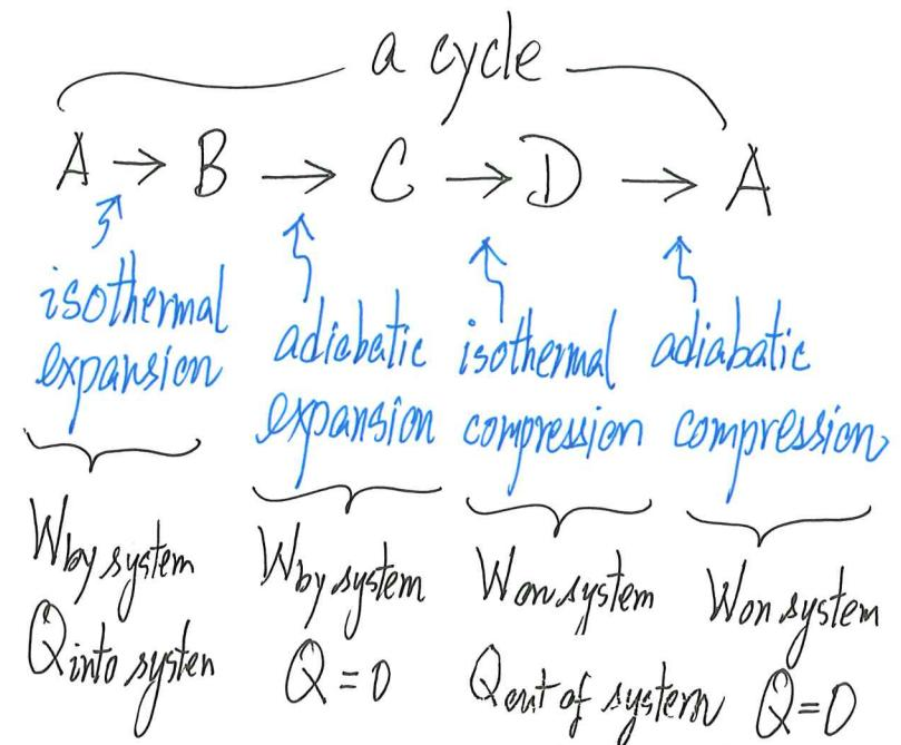
$$\text{Total } W_{\text{by system}} \text{ in 1 cycle} = \text{Area} \neq 0$$
