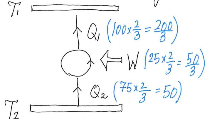
$$\xleftarrow{\underbrace{W' \times \frac{1}{3}}_{\text{part of } W' \text{ to drive Carnot engine backwards}} \left( \frac{50}{3} \right)} \quad \xrightarrow{\underbrace{W' \times \frac{2}{3}}_{\text{remaining part}} \left( \frac{100}{3} \right)} W' = 50$$
